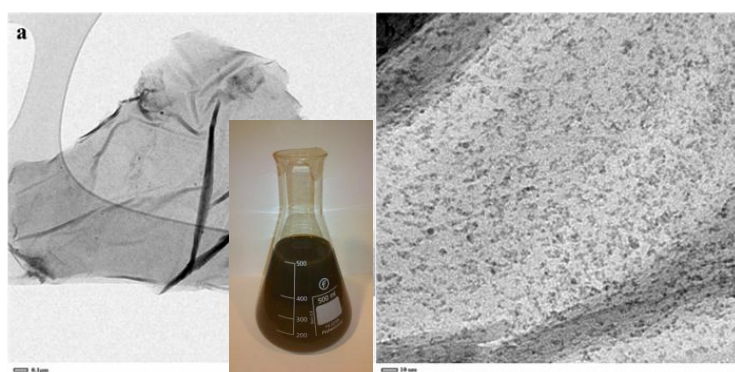
Figure 1 TEM images of SHT GF-AG with different magnifications. A layer of silver nanoparticles with a controlled size of 2~3nm is uniformly dispersed on the surface of graphene.
